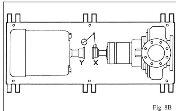
**NOTE:** Failure to slide motor evenly will affect horizontal angular correction.
