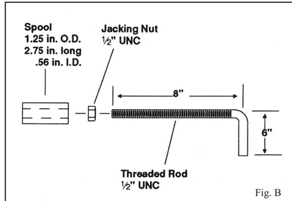
10. Thread jacking nut on threaded rod back about 6 inches (150 mm).
