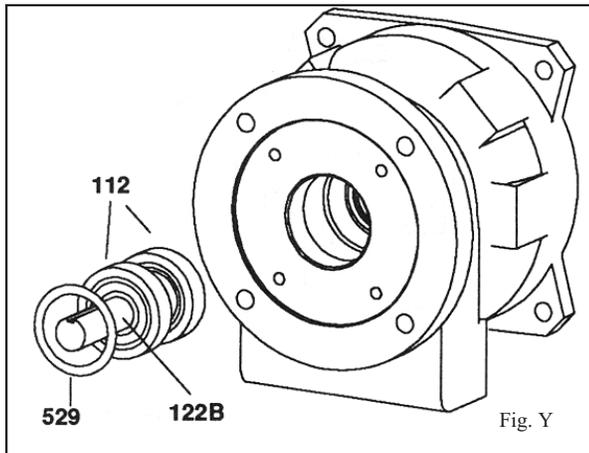
47. Press bearings (112) off shaft and discard.
