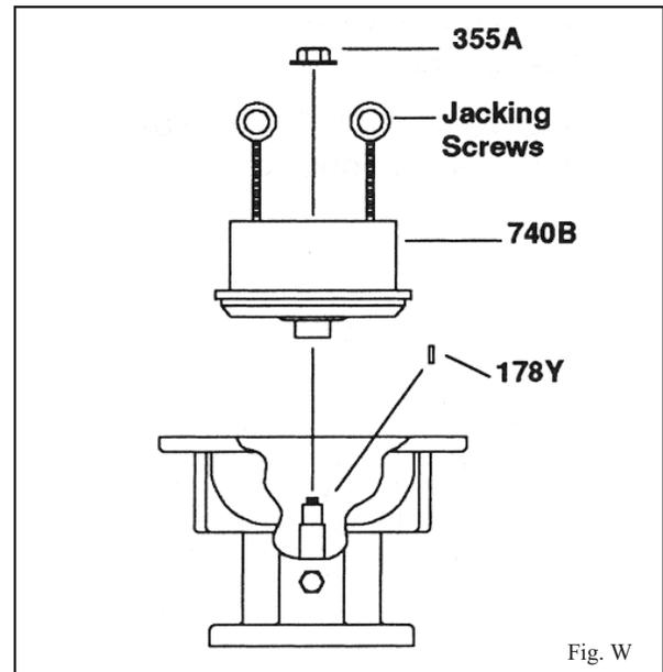
36. Remove drive magnet assembly nut (355A) from shaft (Fig. W).
