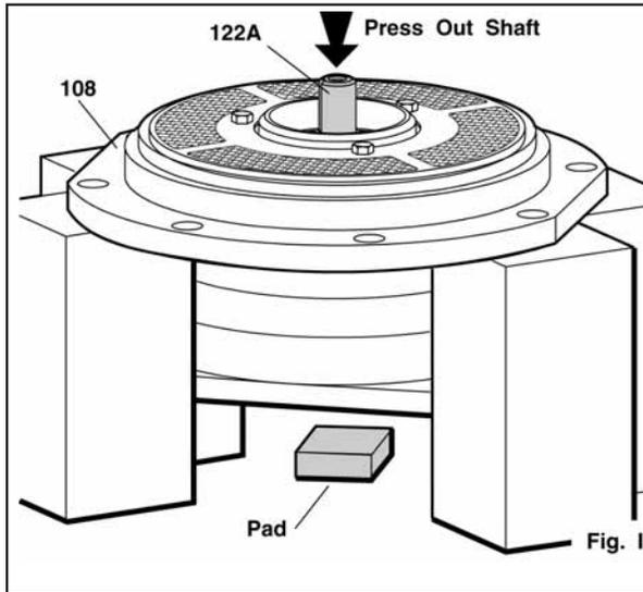
**NOTE:** Outboard rotary sleeve bearing will remain on shaft.
