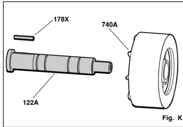
19. Wrap driven magnet assembly (740A) in a clean cloth to keep clean and set aside away from attracting metals.
