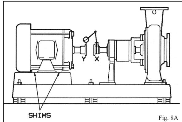
**NOTE:** Equal amounts of shims must be added to or removed from each driver foot. Otherwise the vertical angular alignment will be affected.
