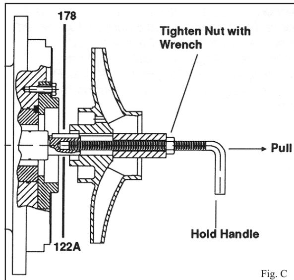
14. Ensure impeller key (178) is in shaft keyway and align impeller keyway to it.
