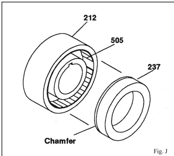
**NOTE:** To ease assembly and minimize the risk of damage to the thrust bearing (237), the use of an arbor press is recommended during installation (Fig. K). Use a small amount of O-ring lube on the tolerance ring and O.D. of thrust collar before assembly.
