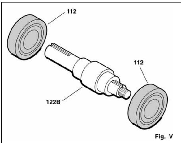
**NOTE:** There are several methods used to install bearings. The preferred method is to use an induction heater that heats as well as demagnetizes the bearings.
